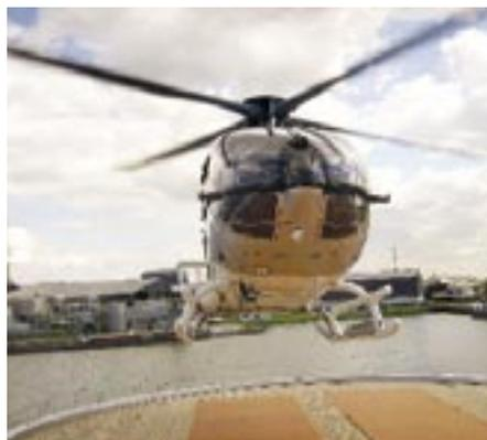
**Helidecks now need to be designed so there is sufficient area to allow the pilot safe access to all parts of the aircraft.**
