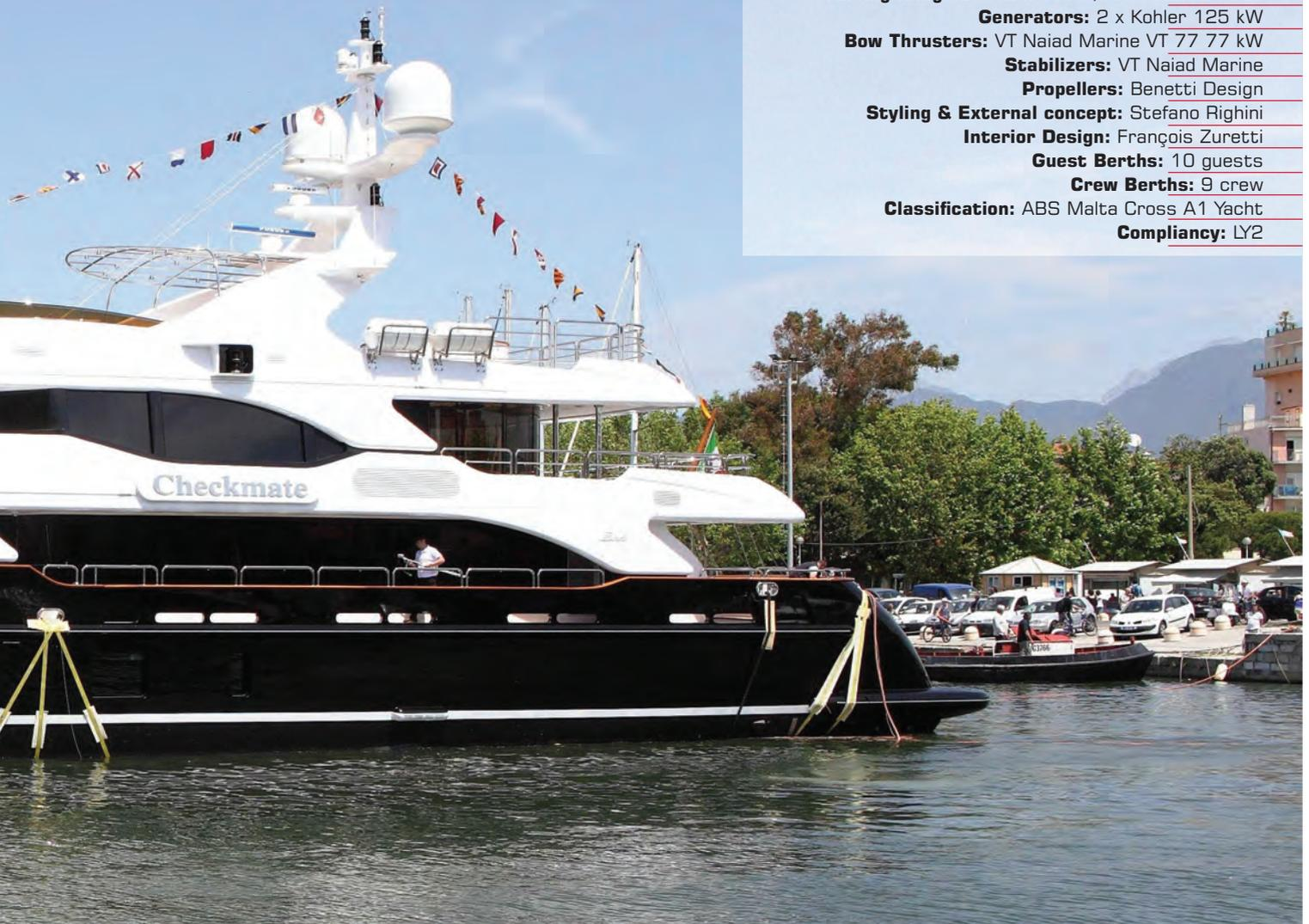
The new yacht is almost 44 metres long with a beam of over 9 metres. Equipped with twin 1,300 HP Caterpillar engines, she is capable of top speeds just shy of 15 knots and at around 10 knots, a cruising range of over 3,500 nautical miles.
