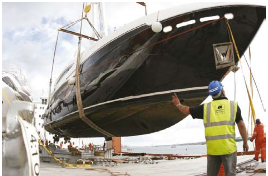
A 37m (121ft) Sunseeker being lowered into a cradle
